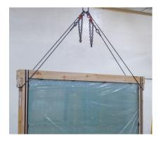
For wood cases handling using a 10,000 lbs forklift boom or 3 Ton overhead crane. Adjustable for  $48" \times 84"$  up to  $96" \times 144"$  cases.
