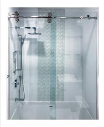
Our popular CLEARWATER Series Frameless Sliding Shower Door Kit offers a modern, low profile design, that includes a round header bar and round glass rollers. It's engineered for use with 3/8" (10mm) or 1/2" (12mm) tempered glazing. Each top glass roller requires one 5/8" (16mm) diameter hole in the glass for proper mounting. Precision bearings and wheels also offer a quiet glide experience.
