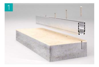
Drill the slab, position the profile and fix the screws.
